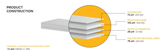
**GENERAL CHARACTERISTICS** TYPICAL VALUES UNIT OF MEASURE **PROPERTIES TEST METHOD** Physical Clearcoat 0.5 etQS005 Film 6.0 mils ± 5% (micrometer) Adhesive 1.1 Liner 3.0 50% Visible Light Transmission TC1800 Tint-Chek Meter Peel Adhesion oz/in 15 minute > 30 PSTC-190 degree 24 hour > 50
